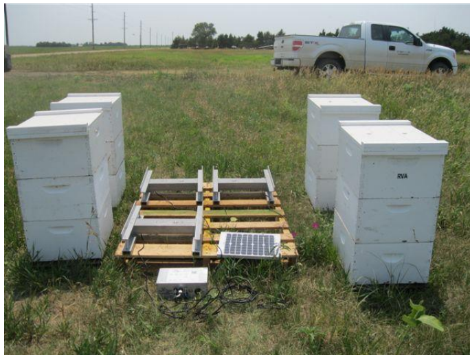
Figure 2: Hive scale data loggers used for study. Pictured here without hive scales.
