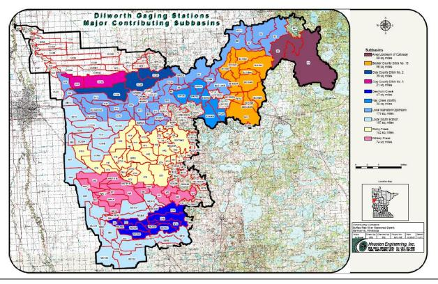
*Figure 10. Spatially Explicit Sub-watershed Priorities for Flood Reduction. Priorities can be identified based on peak flow events associated with the stacked hydrograph data in Figure 9. Finer scale priorities can then be identified based on volume (per sub-basin) and drainage-area-to-volume ratios.*
