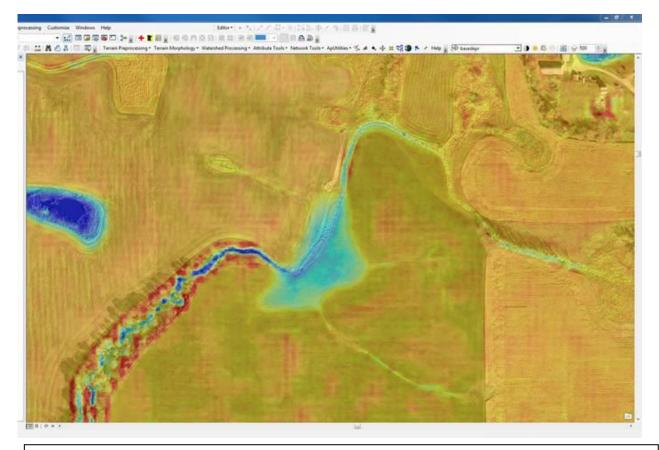
**Figure 12.** LiDAR-derived Drained Wetland Basins. High resolution LiDAR digital elevation data can inform the location of drained wetland basins and provides the basis for the spatial modeling of water volume and nutrient levels associated with individual basins, sub-watersheds, and watershed-scale restoration strategies.
