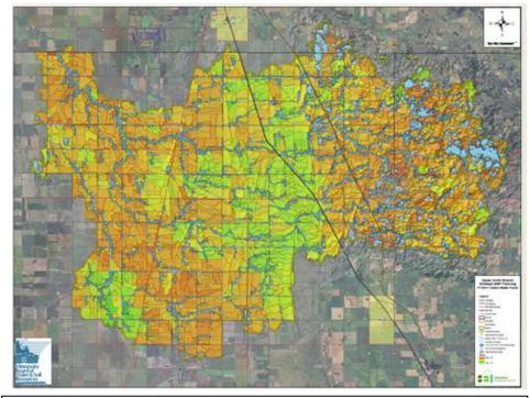
**Figure 11.** An Example of Field-scale Sediment Reduction Priorities. The MN Board of Water and Soil Resources, along with other partners, has worked to develop a process for prioritizing sediment reduction efforts at the sub-basin scale, using LiDAR-derived data.
