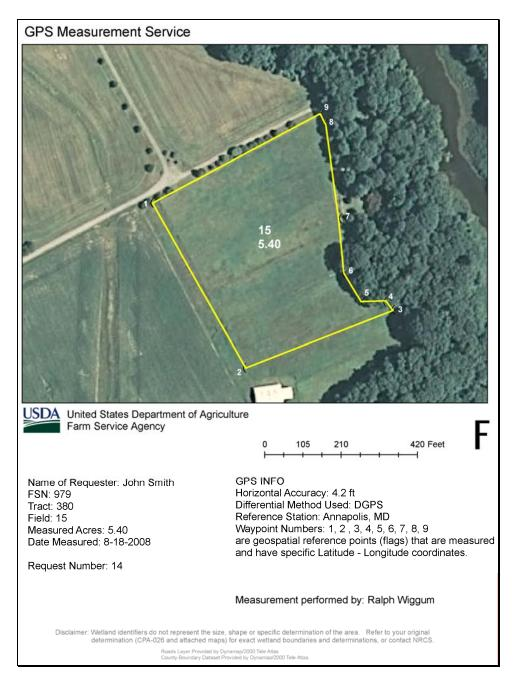
**Note:** This GPS Measurement Service Map Template example can be used for all measurement services. Adding a section of labeled points on the map is optional. The numbered points are GPS waypoint numbers with specific latitude and longitude coordinates.--\*
