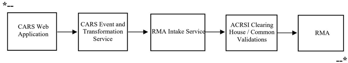
The following is a process flow diagram of the data flow for the AIP Reporting Channel.
