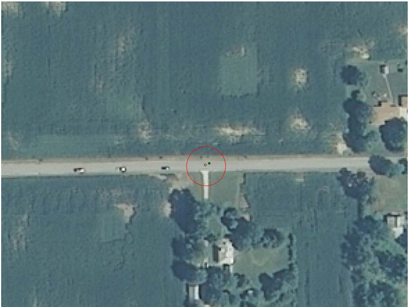
Figure 10: Digitizing a point on the NAIP 2008 image. The green point is the true ground location; the yellow point is the location on the NAIP image.
