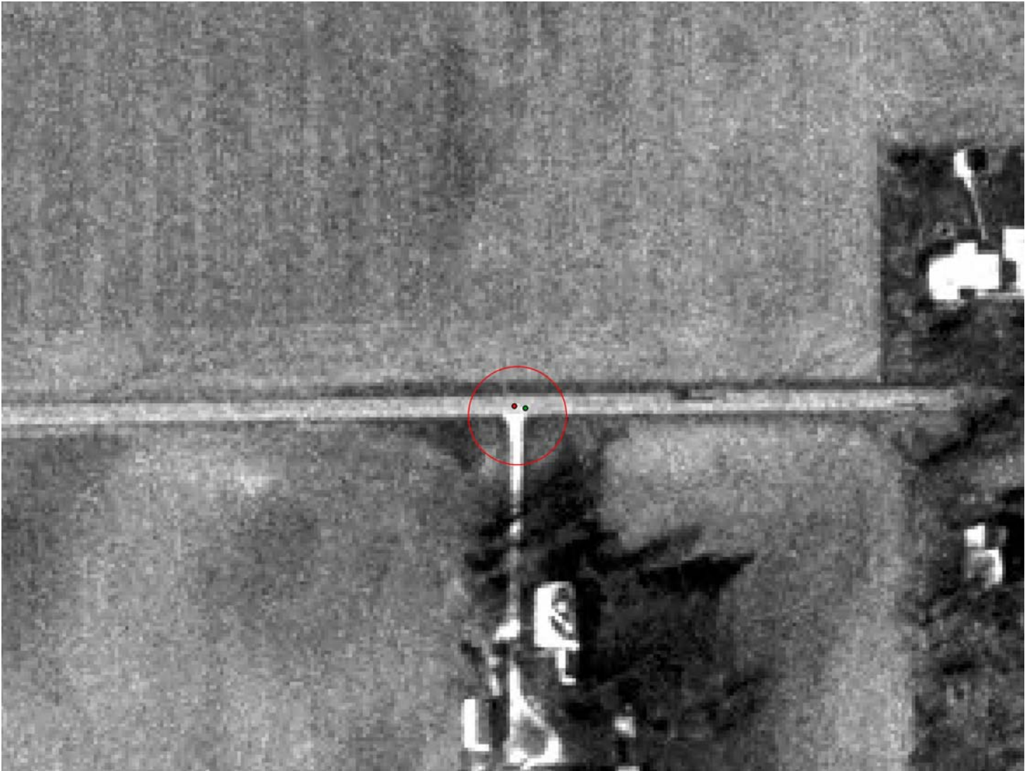
Figure 11: Digitizing a point on the MDOQ image. The green point is the true ground location; the red point is the location on the MDOQ image
