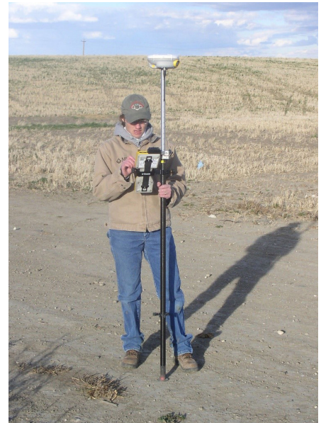
Caption: GPS surveying for Concentrated Animal Feeding Operation (CAFO) project Rimrock Colony West of Sunburst, MT. Oct. 2007. Credit: Montana NRCS
