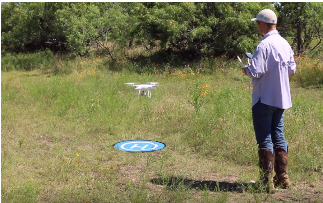
Texas A&M Master Degree student Michael Page operating a UAS and collecting imagery for NRCS project in Tolar, Texas. GEO is examining using UAS technology for detection of invasive grass species in pastures.
